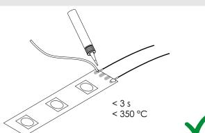
Do not solder for a period longer than 3 seconds. Make sure that the soldering temperature is lower than 350  $^{\circ}\mathrm{C}.$
