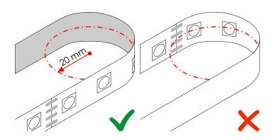
You can bend the LED strip only along the vertical axis. The maximum bending radius is 20 mm. Do not bend the LED strip with the LEDs on the inside.
