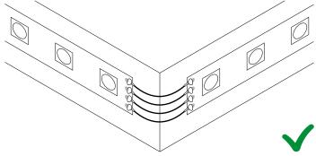
You can also solder wires between 2 LED strips at a corner.
