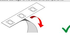
5 Attach the LED strip to the mounting surface or to the aluminum profile.
