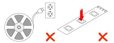
Do not connect the LED strip to electrical power supply when the LED strip is on the reel or when it is tightly coiled. This will damage the LEDs. Do not put excessive pressure on the LED chips.
