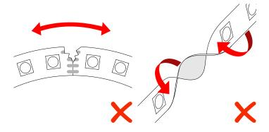
Do not bend the LED strip on the Do not twist the LED strip. horizontal plane.
