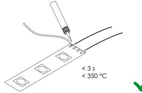
Do not solder for a period longer than 3 seconds. Make sure that the soldering temperature is lower than 350  $^{\circ}$ C.
