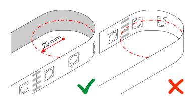
You can bend the LED strip only along the vertical axis. The maximum bending radius is 20 mm.
