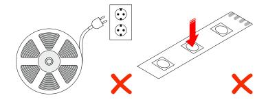
Do not connect the LED strip to electrical power supply when the LED strip is on the reel or when it is tightly coiled. This will damage the LEDs.
